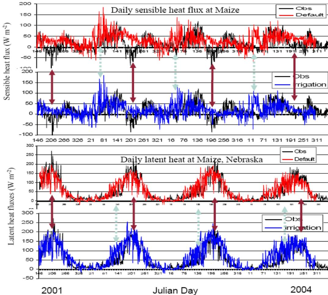
Fig.4a: Sensible heat flux (top two) and Latent heat flux (bottom two) comparisons at Maize (41,16°N, 96.47°W) Ameriflux site, Nebraska. From Top to Bottom, the 1<sup>st</sup> figure is sensible heat flux comparison between observation (dark) and Noah result (red) with default run. The 2<sup>nd</sup> one is
