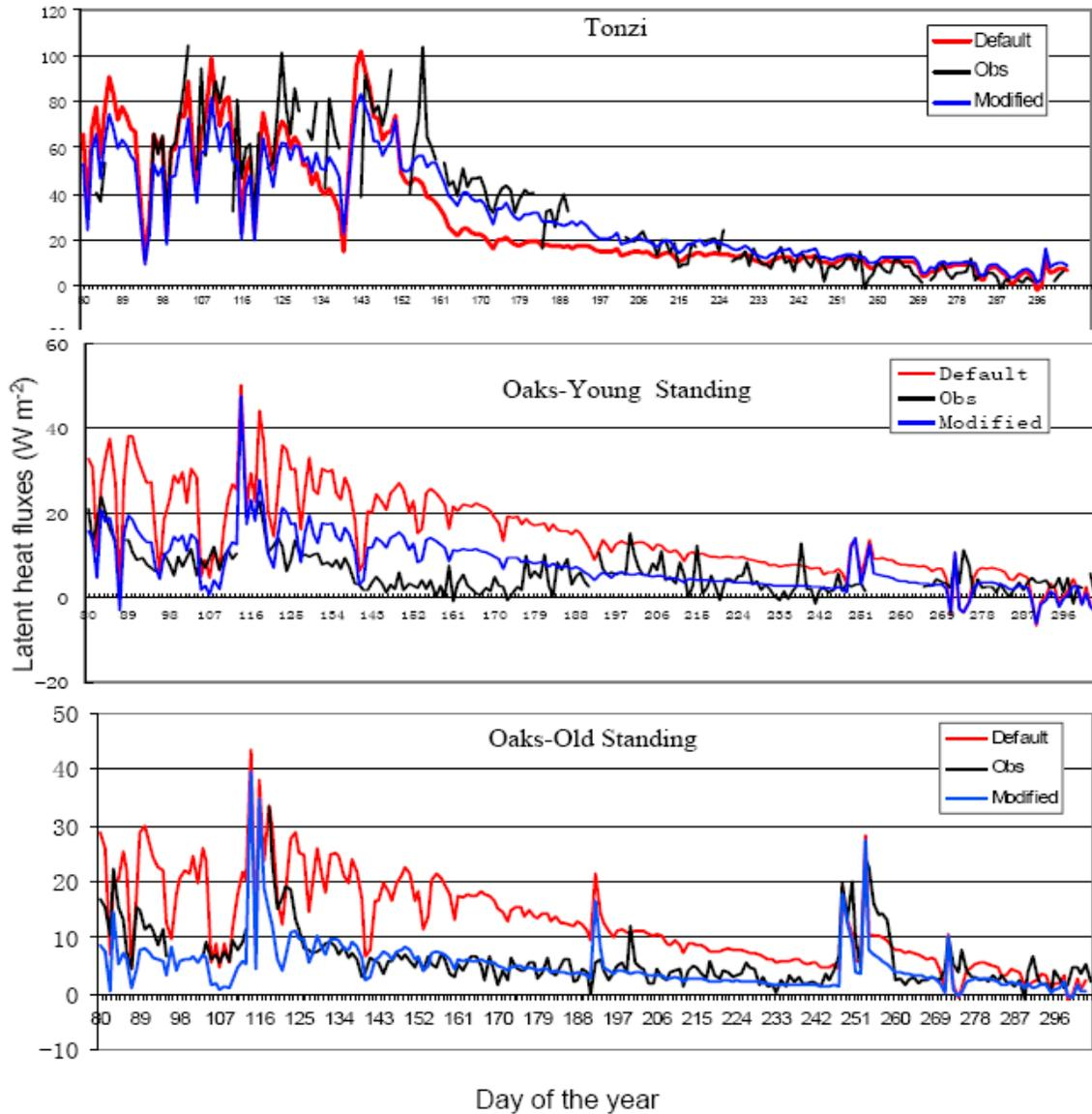
Fig. 2: Latent heat flux comparisons at Tonzi (38.43°N, 120.97°W), Oaks-young- standing (33.377°N, 116.62°W), and Oaks-old-standing (33.37°N, 116.61°W) locations. Dark, red, and blue lines represent observation, model result with default wilting point and model result with changed wilting point.
