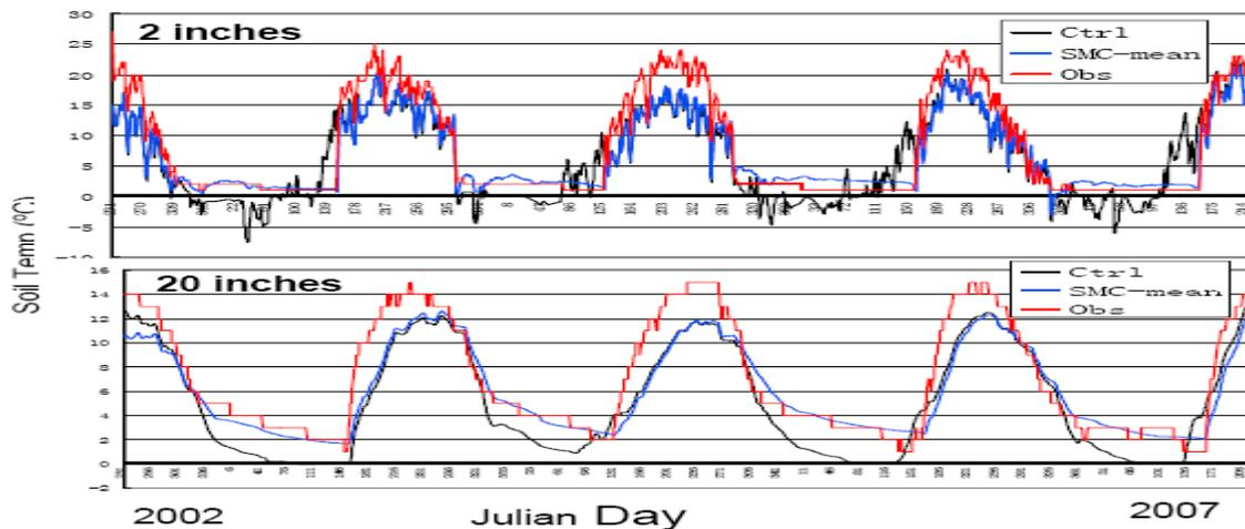
Fig. 6: SNOTEL ID 463 soil temperature comparison between observation (red) and model results with (blue; and sample mean) and without (black) SCA assimilation.
