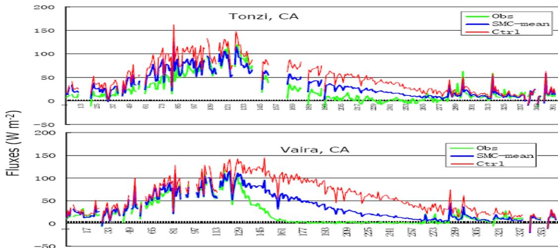
Fig. 5: Latent heat flux comparison between Observation (green) and model control run (red) and the sample mean (blue) with using Sequential Monte Carlo (SMC) method. The forcing data are combined NLDAS forcing and Ameriflux observation. The runs begin Jan. 1, 2006 to May 30, 2008. The date shown in the Figures is from Jan. 1 to Dec. 31, 2007.
