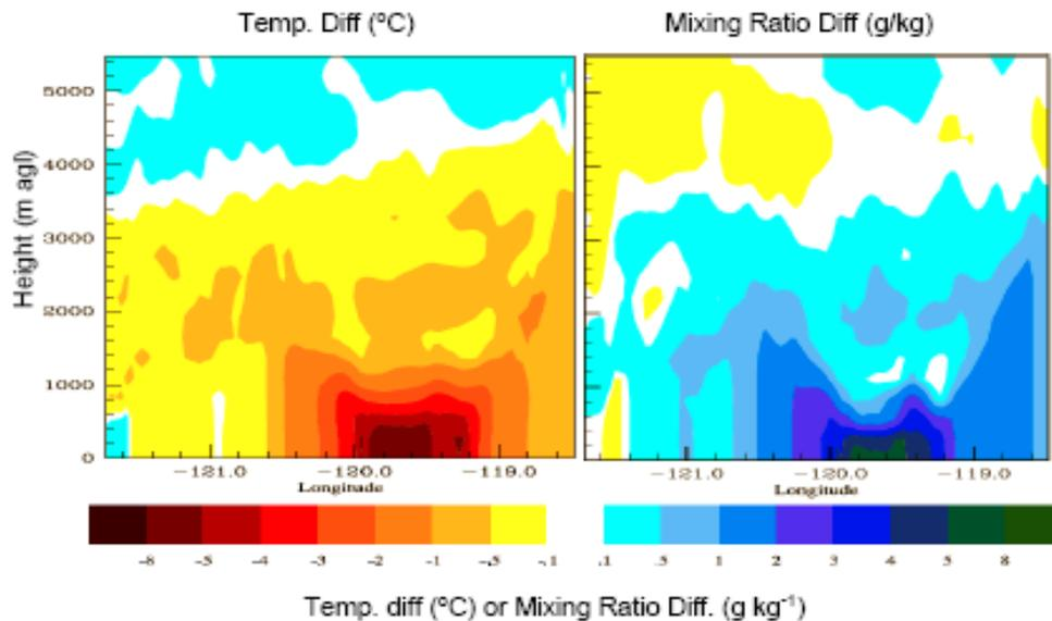
Fig. 14: Cross-section distribution of the difference between irrigation run and control run: left: air temperature (°C), right: relative humidity (%) at 21:00UCT. Data are mean of July 2007. The location of the cross-section is labeled as bold line in previous Figure (Fig. 13)
