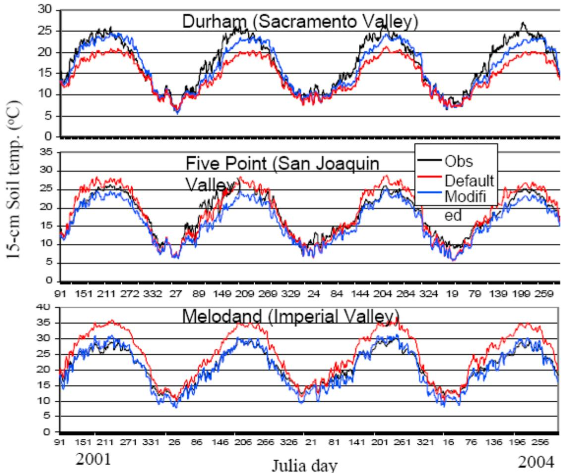
Fig. 3: The comparisons between observation and model results at Meloland, the Imperial Valley. The dark, blue and red lines represent observation, model result with default run and model result with irrigation process added and wilting point changed.
